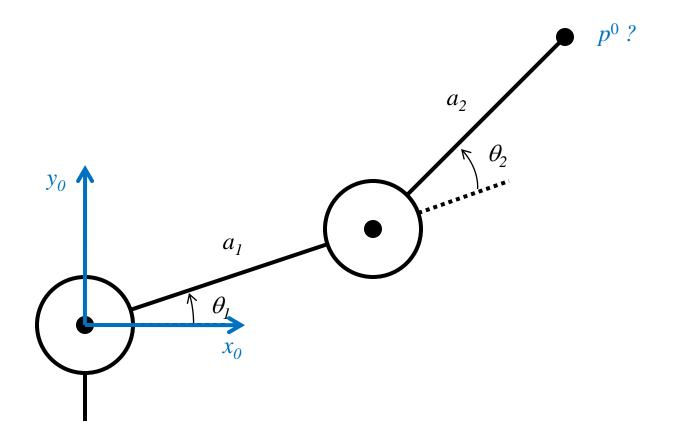
• because the base frame and frame 1 have the same orientation, we can sum the coordinates to find the position of the end effector in the base frame  $(a_1 \cos \theta_1 + a_2 \cos (\theta_1 + \theta_2),$
